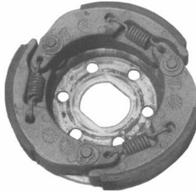
Clutch shoe and spring assembly
